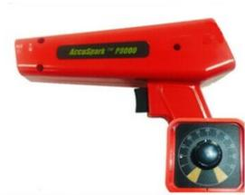
A timing light. If your vehicle has a rev-counter, a simple timing light with an advance control is all that is needed. Although you may prefer to buy the more expensive version that also shows the RPM. If you do not have a rev counter, you will need a more expensive model that shows the engine RPM.
